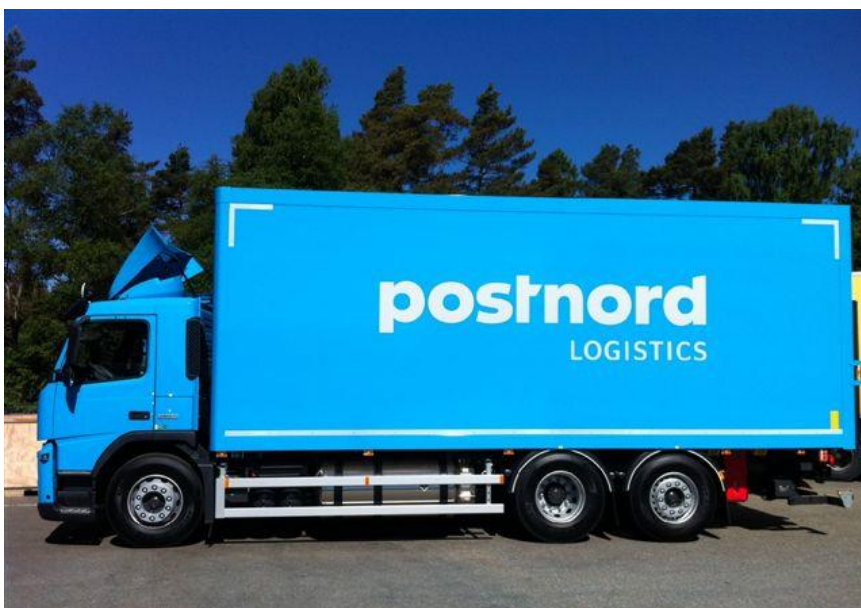
Figure 4. Volvo FM MethaneDiesel truck in operation
