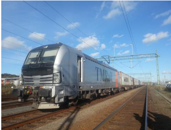
Figure 6, The 722 meter long pilot freight train.
