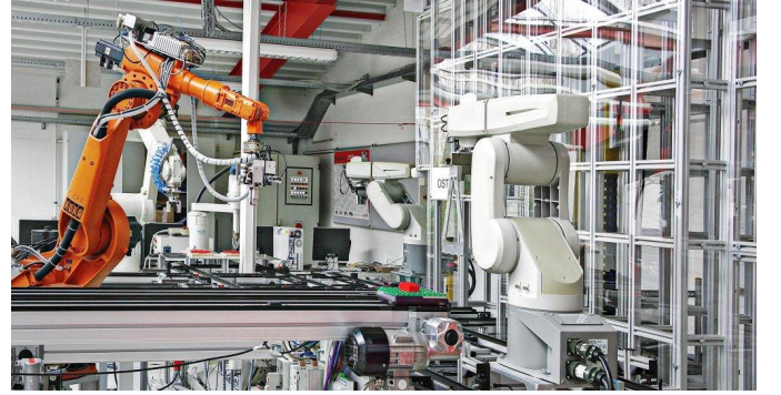
Fig. 7: Test scenario for non-line-of-sight connections in an industrial environment in the Technikum at the University of applied sciences Emden/Leer to arrange comparable conditions such as those on vessels during offshore operations
